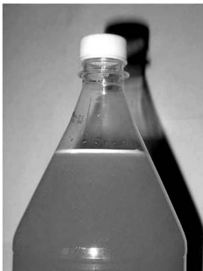
FIGURE 4.1 Neck-ring due to emulsion creaming in cloudy orange beverage.
